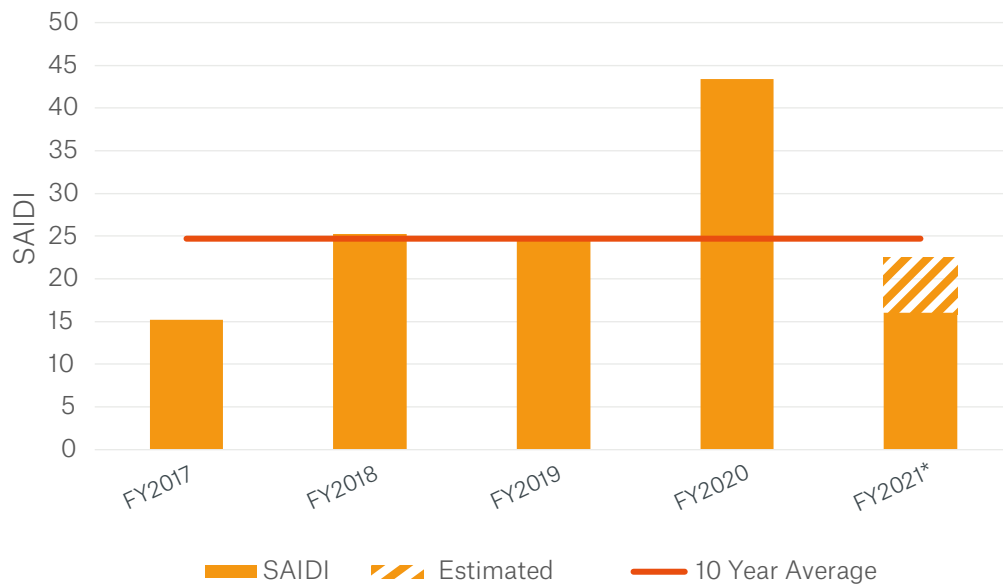
Figure 43: SAIDI minutes attributed to defective equipment annual and ten-year average FY17 – FY21*
