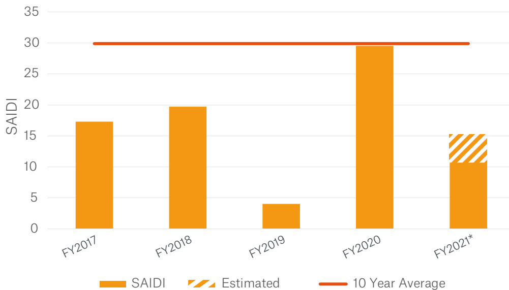
Figure 42: SAIDI minutes attributed to adverse weather annual and ten-year average FY17 – FY21*
